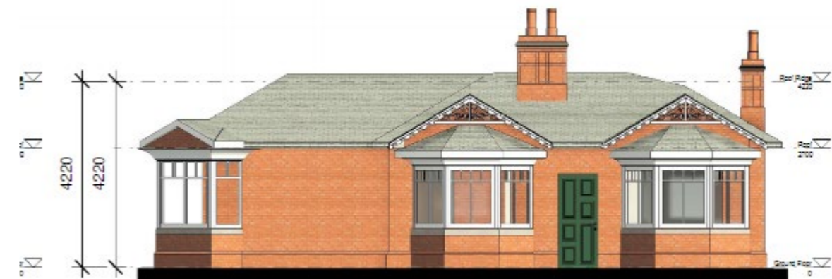
Figure 11.1: North Elevation of Brick Lodge, both chimneys will be retained. (Source: RAU Dwg Brick Gate Lodge , MKS-RAU-ZZ-DR-A-100, Rev P02.)
