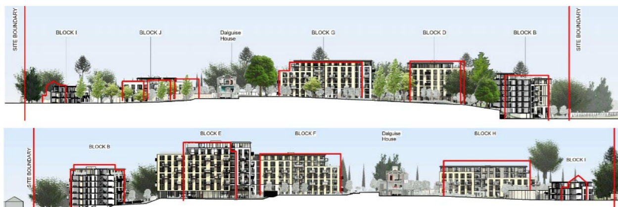
Figure 6.1: Cross Sections of current scheme with the previous scheme outlined in red. (Source: RAU, 2022.)
