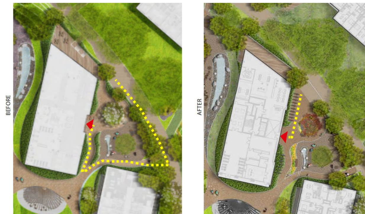
Figure 15.3: Block E pedestrian link between set down area and entrance to Block Planning Application Stage (left) vs Further Information Stage (right). (Source: Cameo RFI Response Report.)
