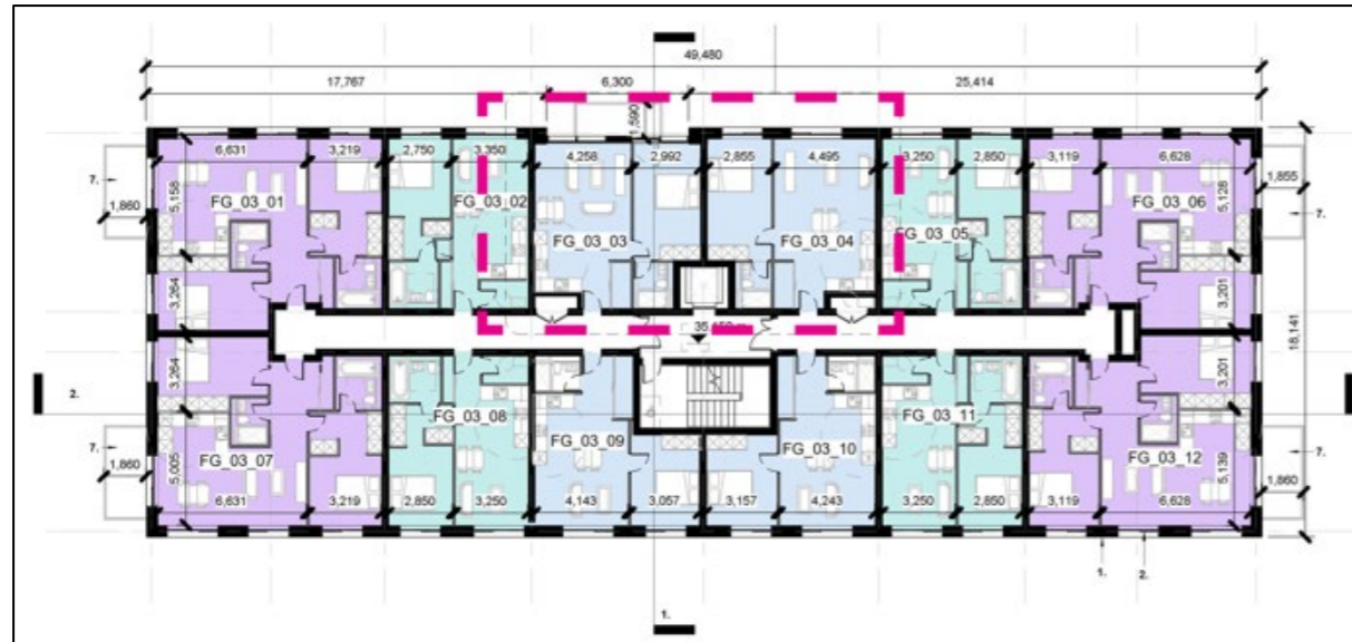
Figure 5.1: Typical Floor Plan of Block H, identifying two adjoining 1-bed units, which could in future be combined to provide a 3 bed unit. (Source: RAU, 2023.)
